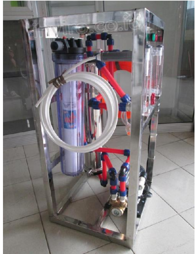
Gambar item no. 1 diatas, Unit Rangkaian Mesin RO (Reverse Osmosis) 1.000 GPD Vontron/CSM (Setara 200 Galon / Hari , 1 Galon = 19 Liter)
