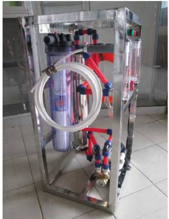
Gambar item no. 1 diatas, Unit Rangkaian Mesin RO (Reverse Osmosis) 1.000 GPD CSM Procon / Rotoflow (Setara 200 Galon / Hari, 1 Galon = 19 Liter)
