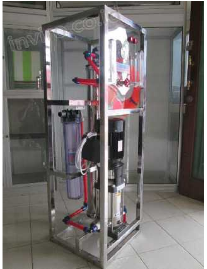
Gambar item no. 1 diatas, Unit Mesin RO (Reverse Osmosis) 2.000 GPD CSM CNP (Setara 400 Gallon /Hari, 1 Galon = 19 Liter)
