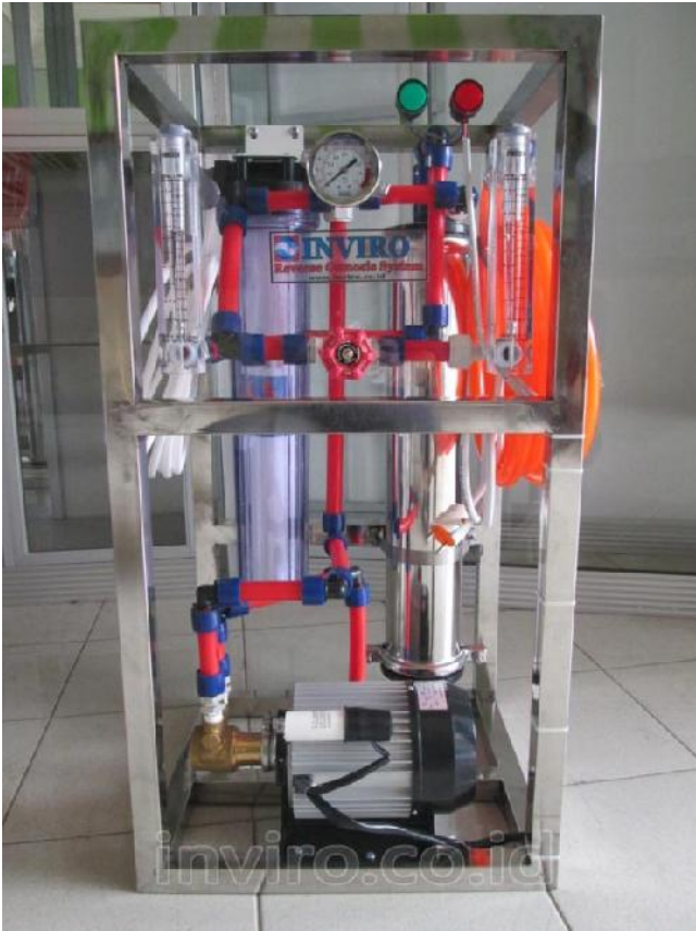
Gambar item no. 1 diatas, Unit Rangkaian Mesin RO (Reverse Osmosis) 1.000 GPD Vontron/CSM (Setara 200 Galon / Hari , 1 Galon = 19 Liter)
